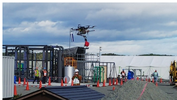
A drone with robotic arm brings the emergency tourniquets in a red bag.
