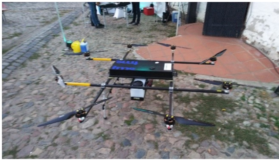
An eight-copter drone used for chemical decontamination.
